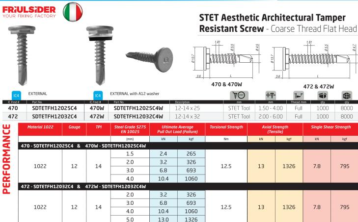
NOTE: Ultimate average pull-out loads for the above screws must be divided by an appropriate safety factor in order to determine either design or recommended loads.
